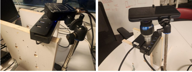
Fig. 3. Recovering a frequency scan using a photodiode (left) and a smartphone (right), by capturing video footage of the power LED of a USB hub.
